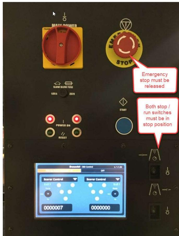
2. Turn OFF both Run/Stop switches before powering up the 360 controller main switch.
