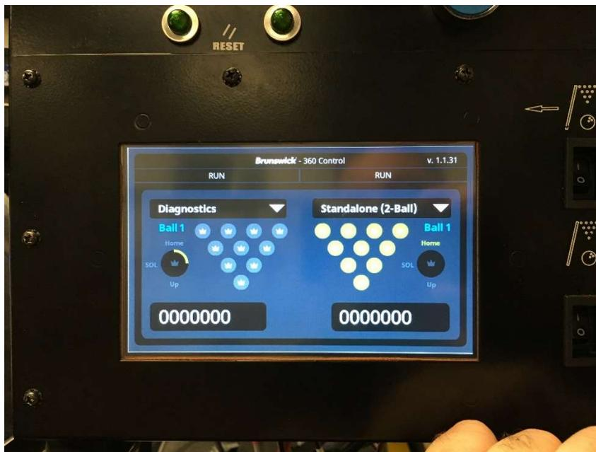
13. After you complete the string brake setup, select Diagnostics from the drop-down menu on both machines and turn them on. Inspect the pinsetters functionality. It should initially set a full rack and then spot pins by pin number order one by one.
