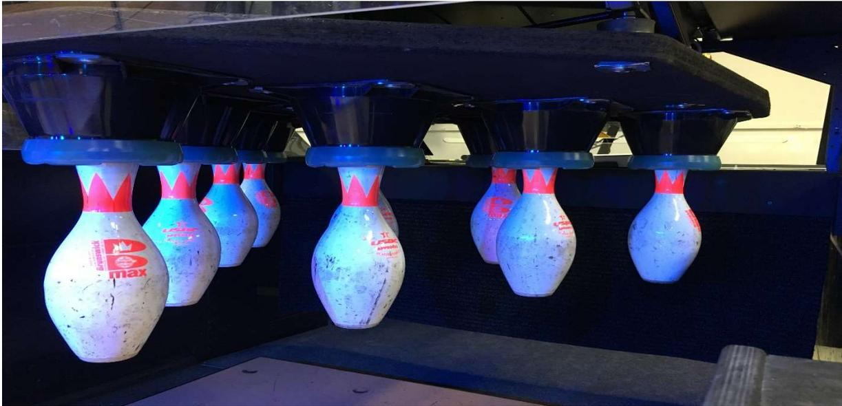
10. Pin solenoid switch will activate the breaks. Notice that the pins are too low in the above picture. Pins 4 to 10 should be showing just the bottom part of the pin crown only.
