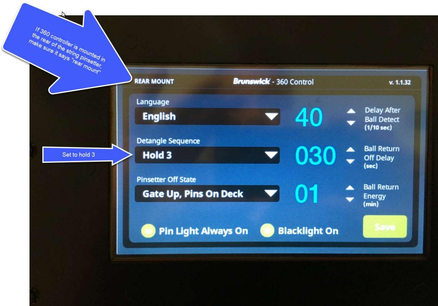
4. Press the Options button on the screen confirm that the above information is correct on your screen and make any necessary adjustments if needed. Press the Save button.
