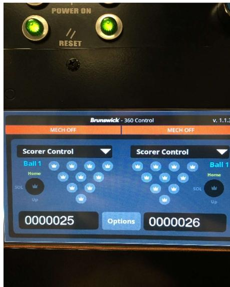
3. After Applying power make sure the two green lights are on indicating the machine is ready to start. If you do not have the two green lights on, please check the emergency stop buttons and check their connections.
