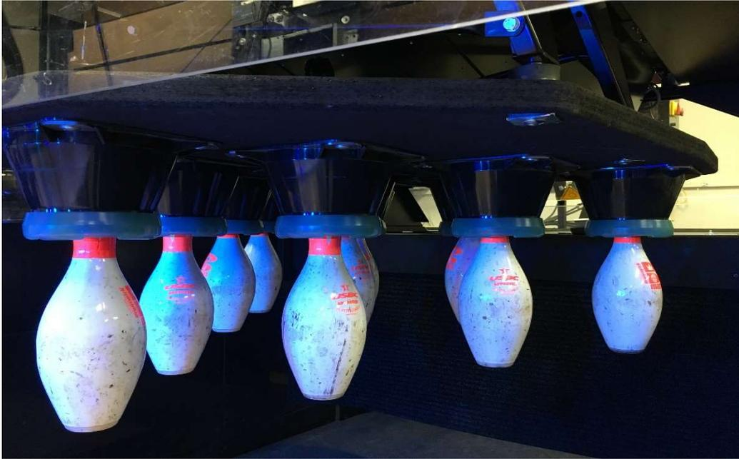
12. The above picture shows the way the pins should look like. Notice Pins 1,2 and 3 will always look lower than the rest of the Pins.
