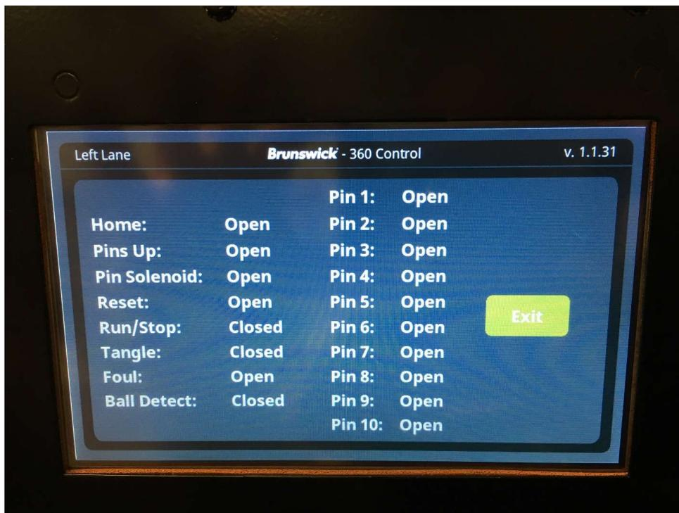
15. You can observe the switch functions in this screen while the machine is cycling. Also, you can test the Pins Motion Interface 'Spics' moving each magnet toward the reed switch. You can now view if the switch for the pin you're testing will switch from Open to Close.
