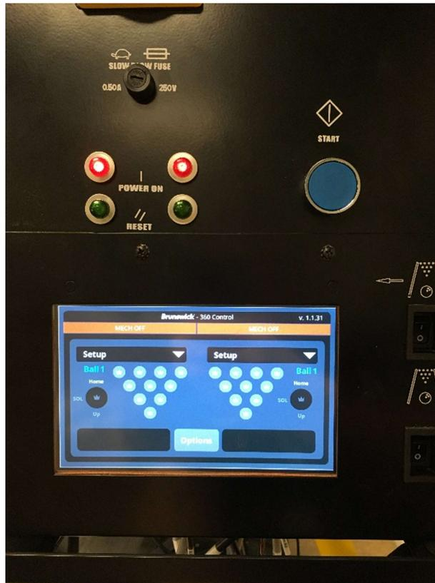
5. Press The blue START button and notice that the status light will switch from green to Red. Switch to SETUP at the 360-controller display and turn both Run/Stop switches into the Run position.
