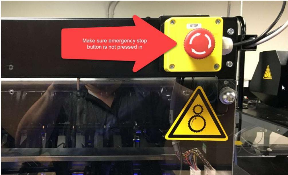
1. Double check that all the emergency stop buttons are not pressed and both are released.
