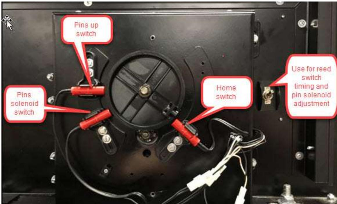
11. To raise the pins to the desired height you will need to adjust the Pins Solenoid switch only. Moving the switch away from the Pins Up switch will lower the pins more. Moving the switch closer to the Pins Up switch will raise the pins. PLEASE MAKE THIS AJUSTMENT MOVING THE REED SWITCH BRACKET IN SMALL INCREMENTS 2MM INCREMENTS TOP. Use the On/Off switch next to the switch cluster to inspect the adjustment.
