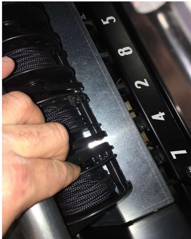
7. Check the string tension by pulling the string to the Arrow direction ensuring that the pin is all the up into the centering cone. Adjust the string reels if needed.
