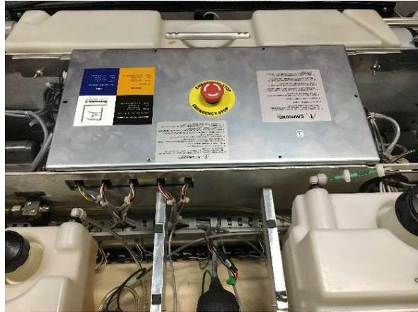
2. Remove the electrical enclosure top cover while ensuring the machine is powered on and the E stop button is not pressed.
