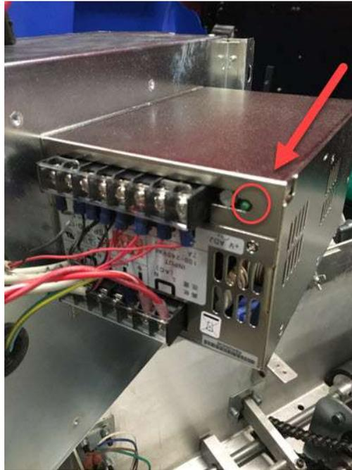
10. Using a voltmeter on AC volts measure the red and red /white cables labeled L and N, the voltmeter should read 120 -130 VAC. If you have 120 -130 VAC reading replace the power supply.
