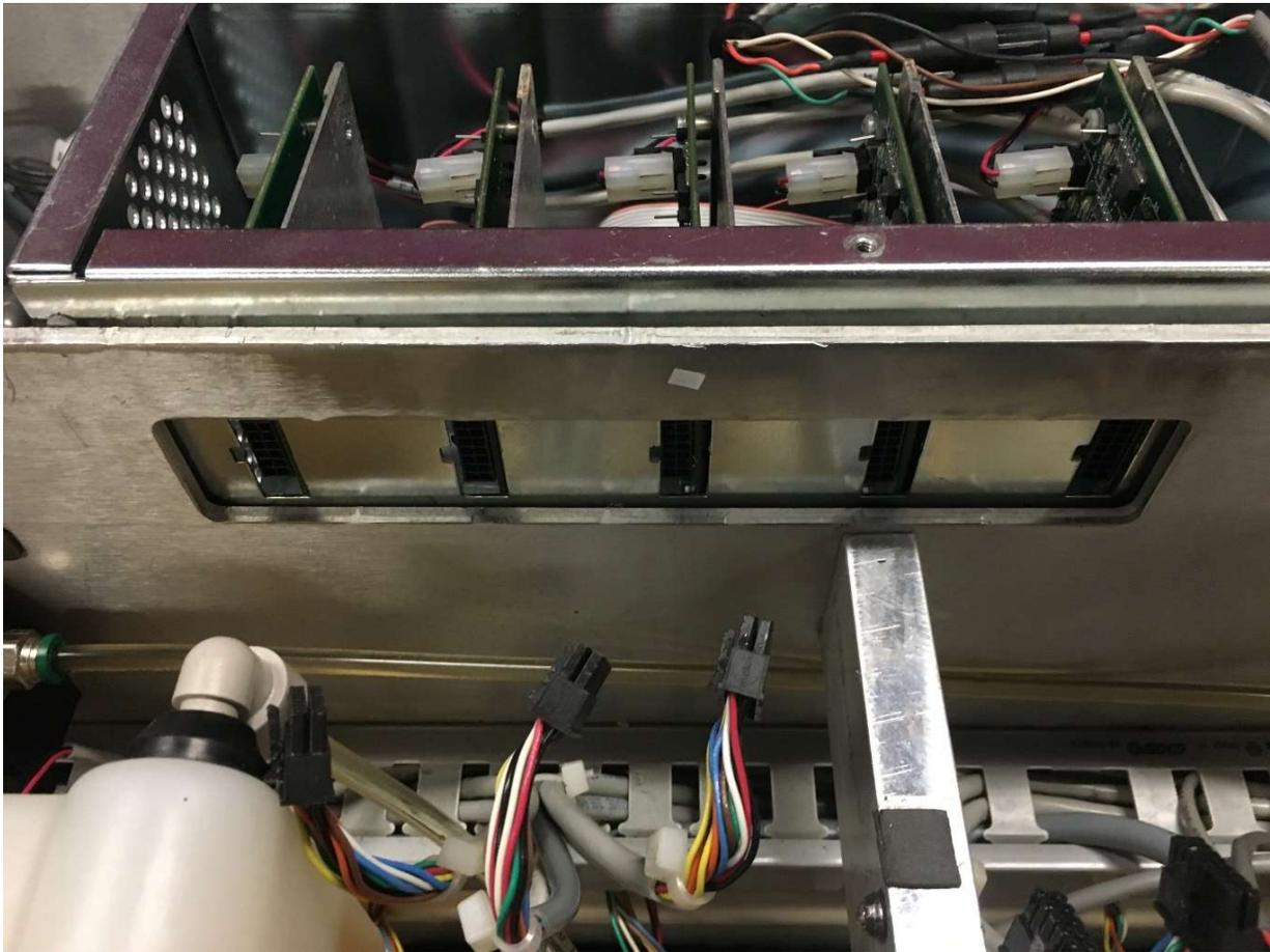
5. Remove the 4 screws that holds the electrical enclosure to the machine main frame.
