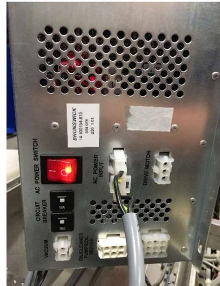
7. Observe at the electrical enclosure power supply. If there is a green LED lit this means 120V is coming from the enclosure.
