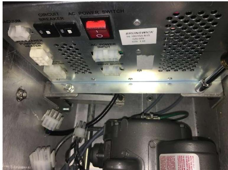
6. Remove the electrical enclosure from the lane machine and place the electrical enclosure sideways on top of the lane machine to access the power supply. Connect the **AC POWER INPUT ONLY.**
