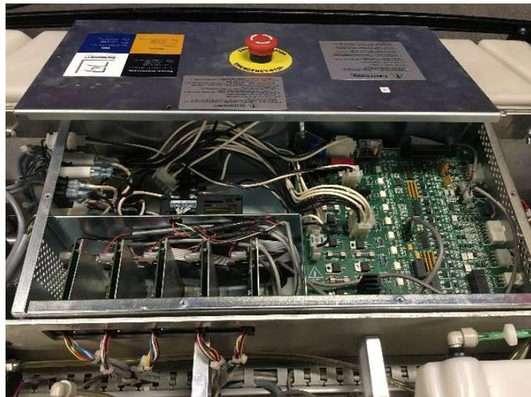
3. Observe if there is any red light lit on the boards. No red LED lights on the boards is a good indication of a 12vdc power supply failure. Proceed to remove the electrical enclosure. Disconnect all the cable connectors from both sides.
