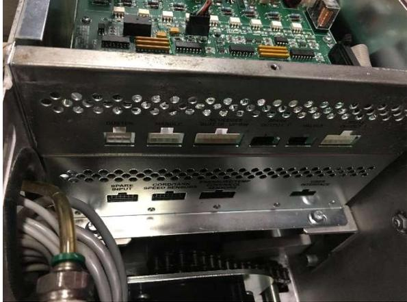
4. Disconnect the injectors control cables.
