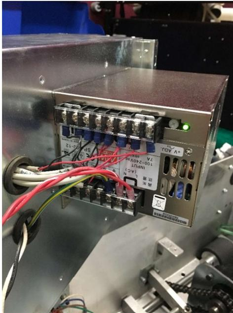
8. Using a Voltmeter set to DC volts, measure from any red and any black wire from the output section. If it's lower than 12VDC use the adjustment pot to increase voltage.
