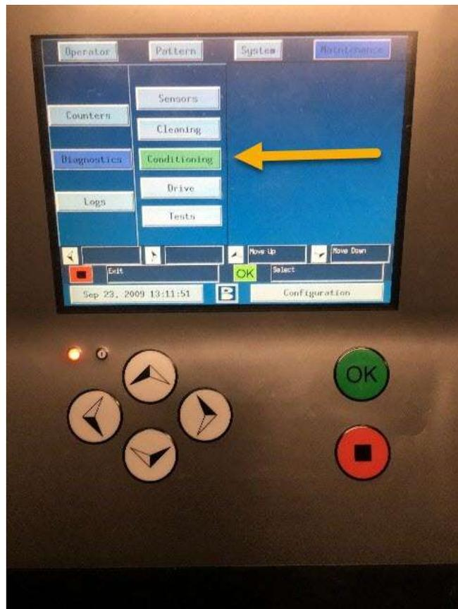
2.) Activate the Oil Pump and press the stop button when it reaches above 20 PSI.
